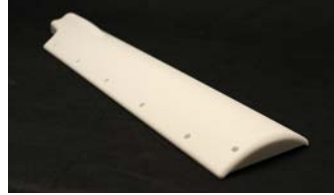
Figure 2: FDM pattern for silicone molding.
