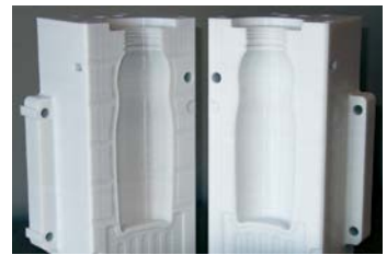
Figure 8: FDM blow molding tool made from polycarbonate.
