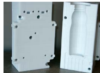
Figure 3: Polycarbonate blow mold made from the FDM process.
