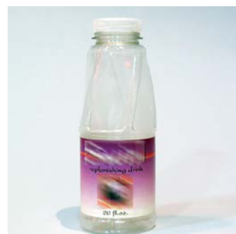
Figure 4: Prototype bottle molded in PET.
