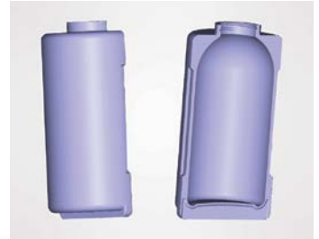
Figure 10: CAD data for a contoured insert that is mounted in a machined mold base.
