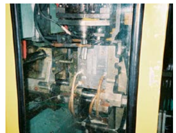
Figure 13: Prototype hybrid FDM tool mounted in blow molding machine.
