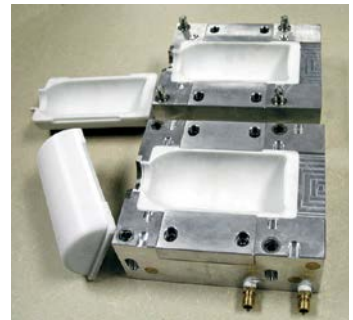
Figure 9: FDM hybrid tool with contoured inserts.
