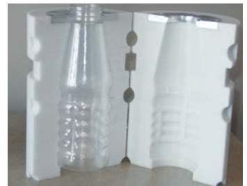
Figure 11: To mold the PET bottle, this hybrid insert uses a cylindrical design.
